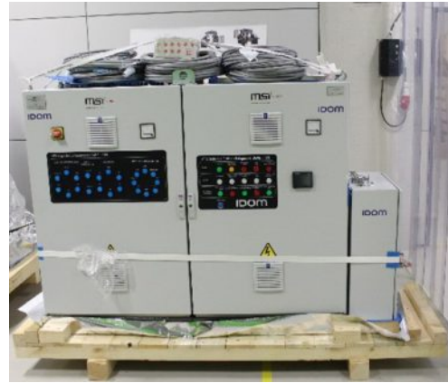
Packing of the electrical cabinets for transportation
