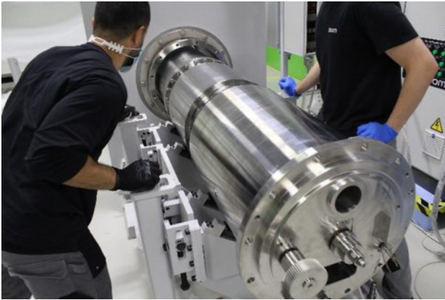
Assembly of the collimator system onto the test nozzle
