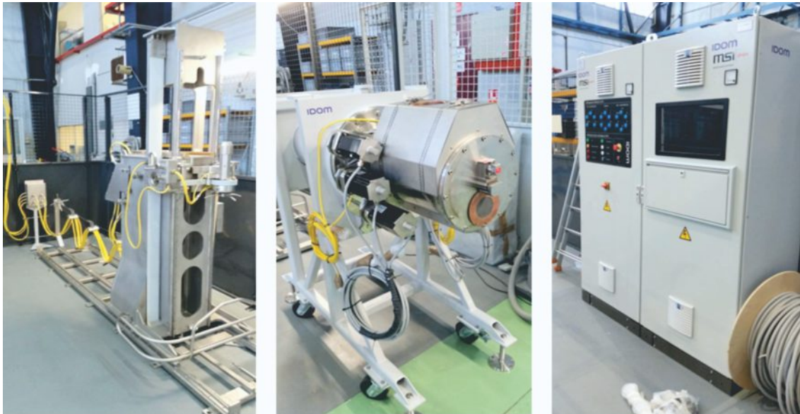
HGXR devices assembled at Cadarache (Totem hall) The hot cell bench on rails (left), the gamma collimator system with detector shield (middle), and the electrical cabinets (right).
