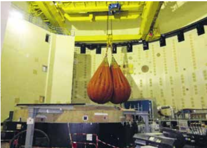
Loading tests of the polar crane
