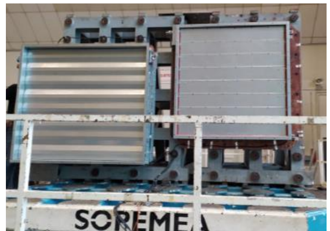
Qualification of ventilation damper used in the safeguard buildings
