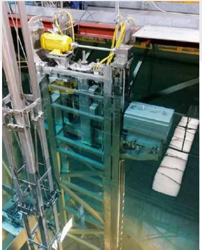
Tests on the EMI conveyor in water (seizing problem revealed)
