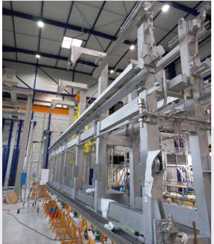
Tests on the EMI conveyor in water (seizing problem revealed)
