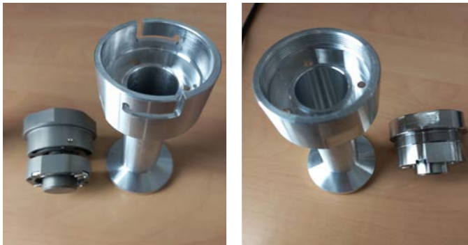
Figure 1: Bayonet and screw-type locking systems tested
