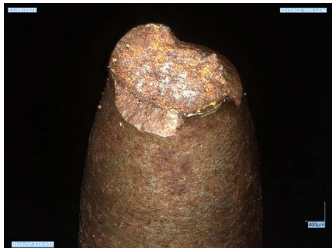
The fracture surface of a traction specimen reconstructed from data collected by a hot-cell non-destructive test bench (digital macroscope)
