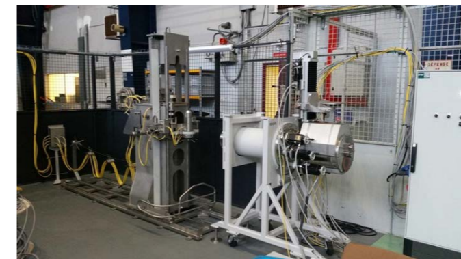
Hot cell bench and collimators in the TOTEM facility
