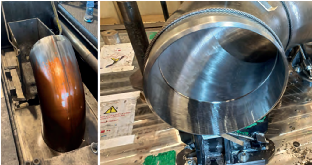
Extrusion of the elbows of the primary circuit
