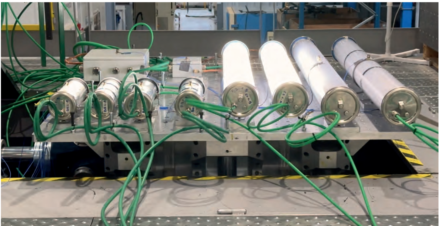
Earthquake testing : light projector and flame / smoke detector
