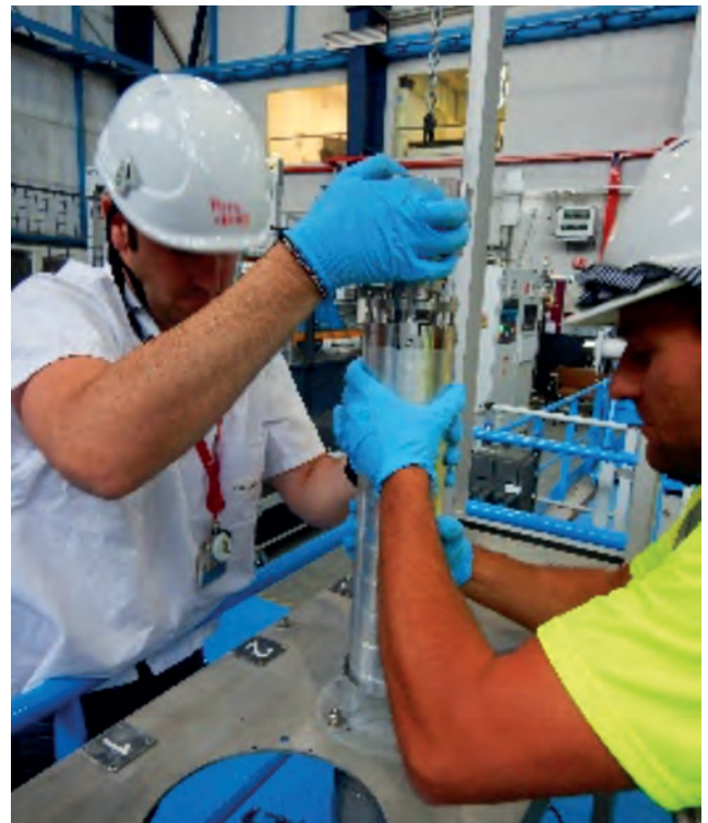
Introduction of PROSPERO model in the CORALIE hydraulic loop
