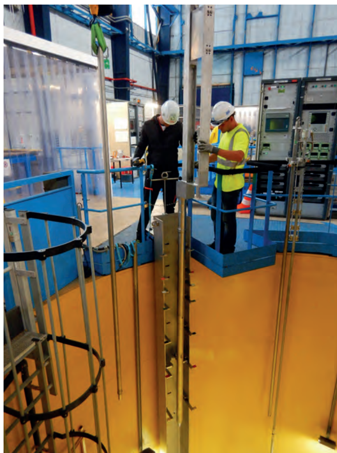
Docking test of an experimental device on the work table in TOTEM pool
