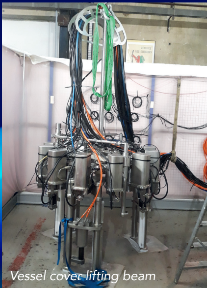
Conditioning of the vessel cover lifting beam in 20-foot containers
