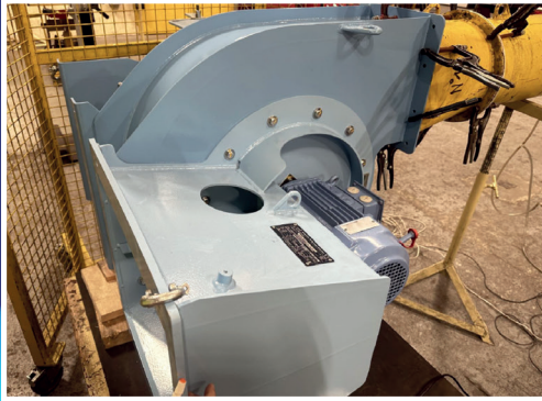
Factory acceptance of the exhaust fans
