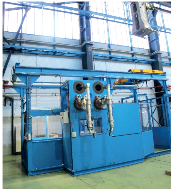
Installation of the HGXR bench inside the mock-up of JHR hot cell in TOTEM facility
