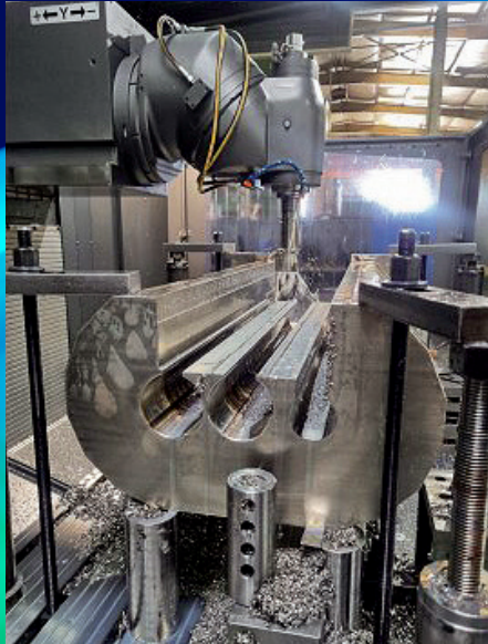
Machining of the frame for the ex-core measurement system
