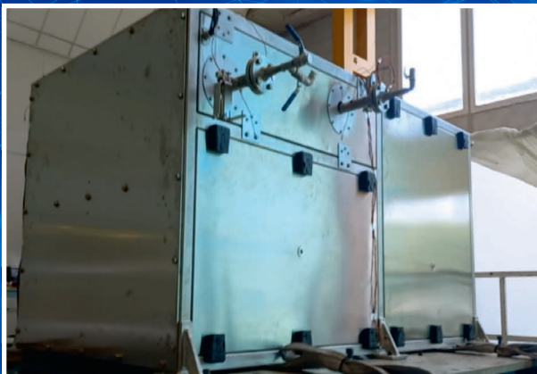
Seismic test for Prototypes of safety-relevant Local Air Coolers
