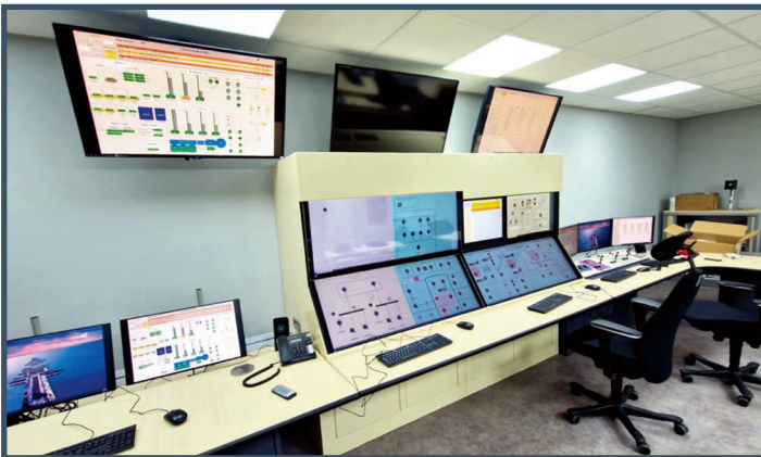
JHR simulator will be used to model the physical phenomena of main circuits, to define reactor operating procedures, and to train future operators
