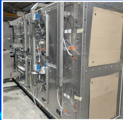
Factory acceptance of Air Handling Units
