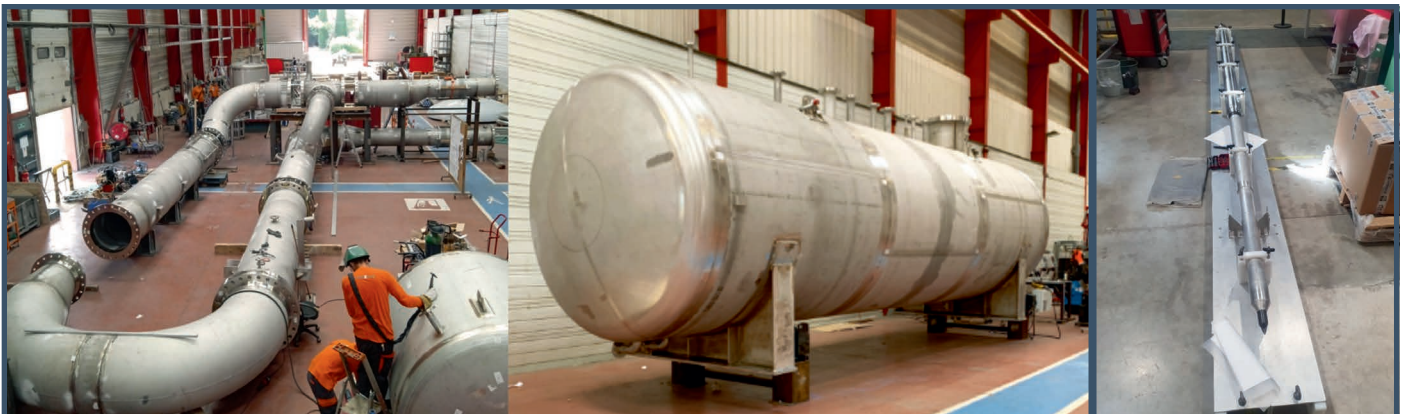
- Experimental test section (left) installed in BMM (pump to be installed) with its water tank (center)
