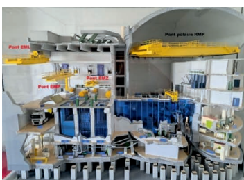
Auxiliary building cranes
