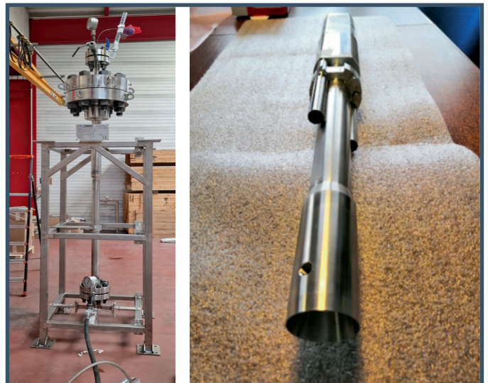
Flow test section (without thermal shroud) & flow amplifying module
