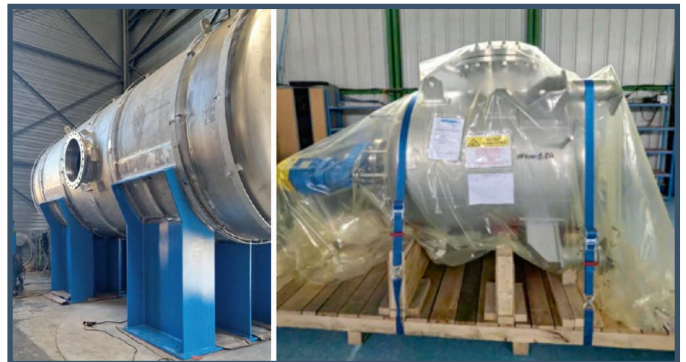
Reservoir for the safety cooling system devices
