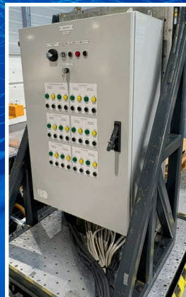
Seismic test for Prototype of fire dampers cubicle
