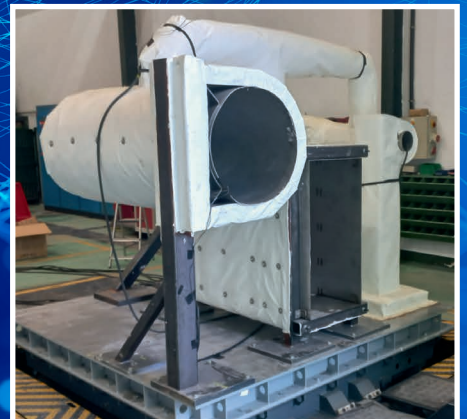
Seismic test of ductwork fire protection
